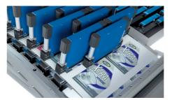
Micro-motor controllers precisely align each print head – creating a seamless image across the corrugated sheet to deliver the high print quality results.
