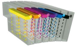
Ink circulation provides consistent print results and the optimum reliability - maintains a constant temperature and removes micro air bubbles enhancing ink jetting stability.
